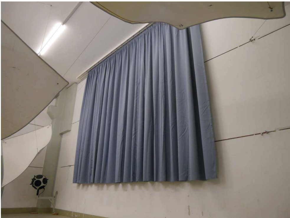
Figure B.2. Test arrangement in the reverberation room (diagonal view).
