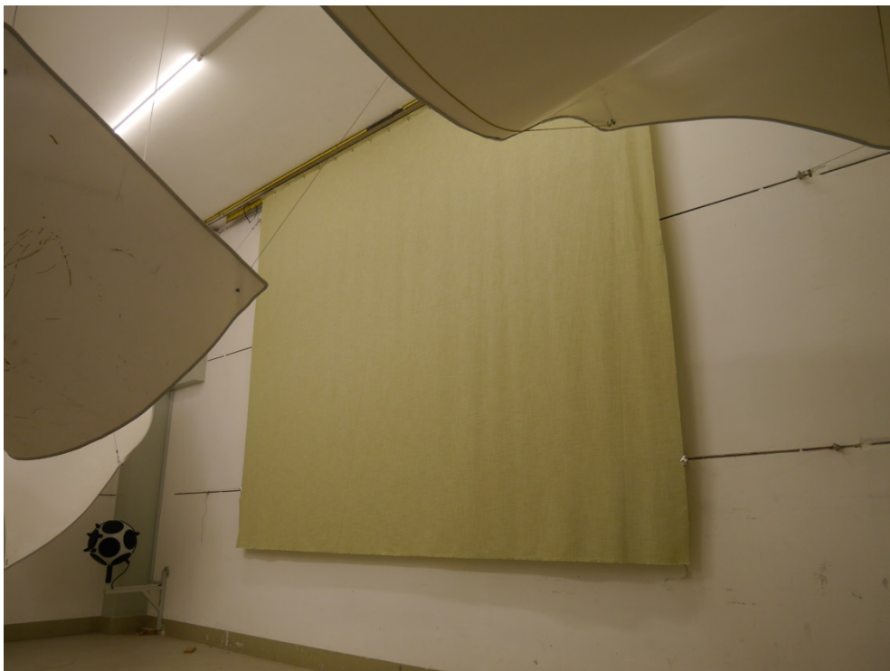
Figure B.2. Flat arrangement: test object mounted in the reverberation room, diagonal view.
